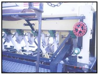
**Photo 2.3.** Addition of a crank wheel to improve accuracy and ease of calibration.
