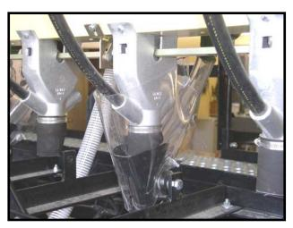
**Photo 2.4.** Addition of windshields to reduce seed loss during windy conditions.
